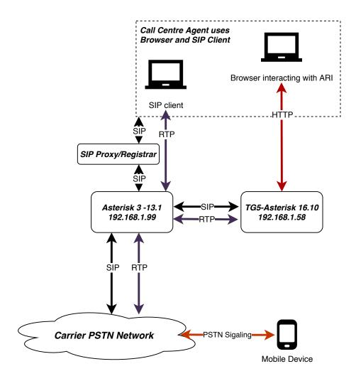
RTP Flow To show where we see the issue between Asterisk 3 and TG5 Note Asterisk 3 is the edge device to carrier and SIP client for signaling and media streams involved in this issue. Note IP addresses and ports will match debug and wireshark traces - I have tried to simplify with just showing RTP and not SIP when silent RTP packets are sent. Note legs to Carrier and SIP client are not shown as issues occurs on TG5 as will be seen from wireshark traces. Issue only occurs when recording.
