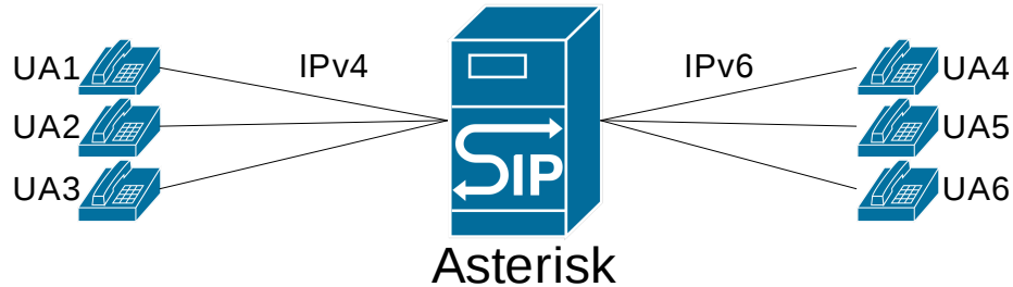
Figure 1: Test setup comprising three IPv4 user-agents, three IPv6 user-agents, and a dual-stack Asterisk server.
